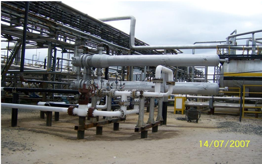
**Fig.2 3S-separator at Gubkinskoe CGTP, JSC "Rosneft"**
